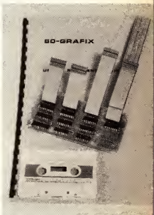
The kit is comprised of the built up circuit board, the instruction manual and the cassette tape containing demonstration programs.
